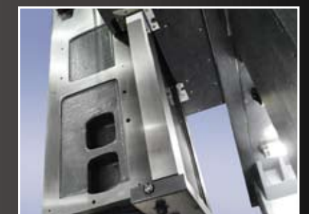
■ Hardened and Ground Box Guideway on Z-axis (DCV2012B)
