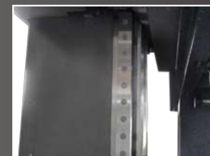
■ Roller Type Guideway on Z-axis (DCV2012A)
