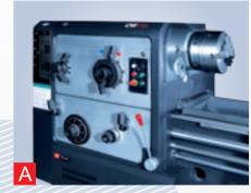
**Headstock** High torque and high speed in the same package. The spindle forward speed ranges from 5.4 to 720 rpm with 18 speed settings. The highly rigid spindle offers a maximum torque of 2233 Nm.
