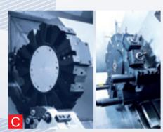
Turret Our standard configuration is a 12-station hydraulic turret from Taiwan. This design is driven by a hydraulic motor and features high reliability and rigidity with minimal deformation under heavy-duty cutting. Certain models offer live tooling for use as turning centers. Turret height can be from 160mm to 200mm according to customer need.
