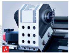
optimizations have been made to improve manufacturers. spindle accuracy and rigidity. The spindle has been ground tighter with the inner bearing ring while the headstock has been bored tighter with the outer bearing ring. The spindle bearings are pre-tightened. Some series models feature a variable-speed spindle headstock.
