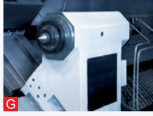
Tailstock Driven by automated hydraulic control, our tailstocks come equipped with high precision bearings from NSK. The end result is excellent rotational accuracy and very high rigidity. An optional hydraulic locking mechanism for the tailstock sleeve is available to eliminate cutting-induced vibrations.
