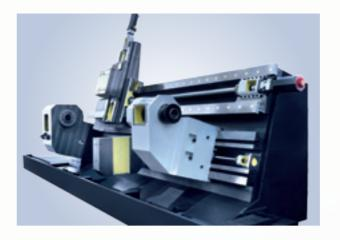
From the 45° and 75° integrated slant beds to the specialized spindle, bed, and tailstock design, each aspect of this series has been optimized for overall rigidity. Excellent stability can be expected even during high-speed heavy-duty turning.
