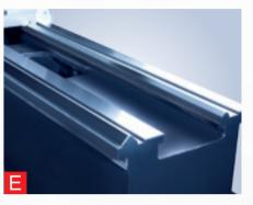
Guideway The flat bed guideways are heat treated and hardened to a depth of 3mm and rating of HRC52. The saddle and sliding guideway surfaces are Rulon-coated for smoothness and durability.
