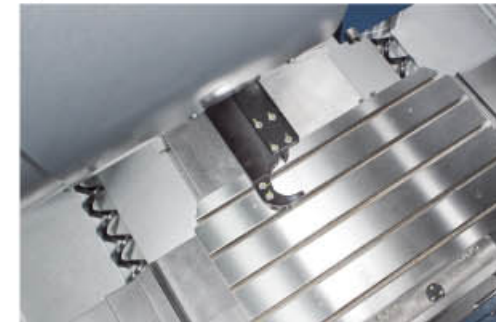
Twin Chip Augers Chip Augers are deployed on the two sides of machine base to evacuate cutting chips efficiently.
