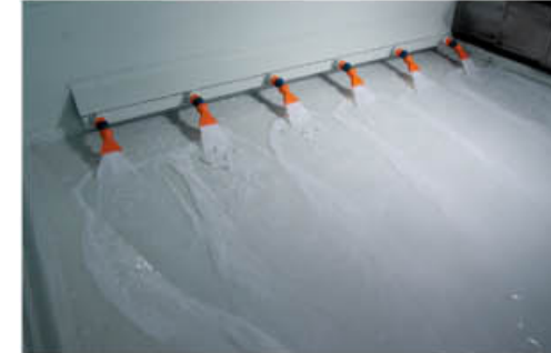
Chips Flushing Nozzles Coolant flushing nozzles on rear inner wall of guard prevent jam of chips during operation.
