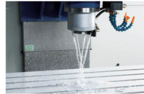
Coolants Jets Around Spindle Improved cooling efficiency on workpiece.
