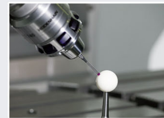
Kinematic Opt. (Option) Kinematics Opt is an important component to help you meet these high requirements: With a HEIDENHAIN touch probe inserted, a 3-D touch probe cycle measures your machine's rotary axes fully automatically. The results of measurement are the same, regardless of whether the axis is a rotary table, a tilting table or a swivel head.
