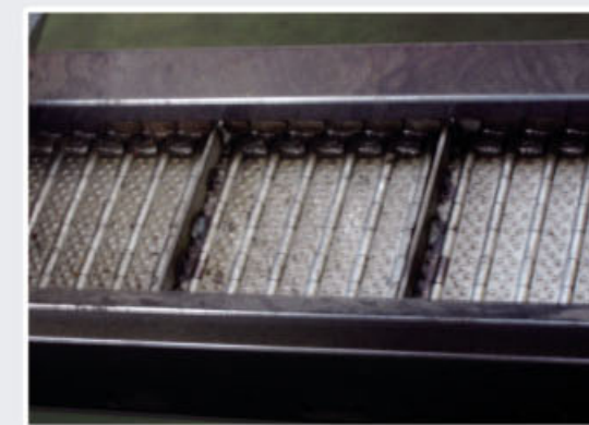
Chip Conveyor (Option) Hinge type or scraper type chip conveyor in front side of machine (able head to left or right) removes chips from machine.
