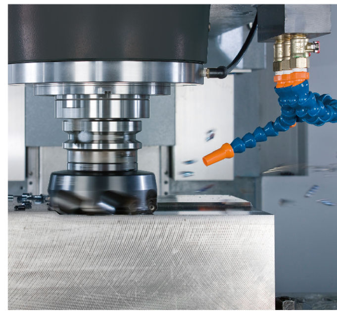
It is designed for heavy cutting with high removal rate over 500cc/min in S45C material.
